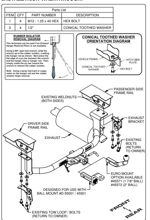
1. Remove existing bolts from rearmost exhaust hanger to lower exhaust. Return bolts to owner. **NOTE:** For ease of installation rearmost remove rubber isolator. See RUBBER ISOLATOR REMOVAL DIAGRAM.
