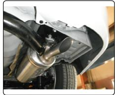
5. Torque all 12mm fasteners to 86 ft-lbs.
