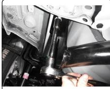
Reinstall rubber isolator (if it was removed in step 1).
